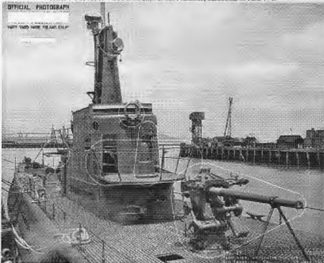
Photo taken at San Francisco, California, 13 June 1943, at the conclusion of an overhaul in the Mare Island Navy Yard, California. Circles mark recent alterations, including a 3"/50 deck gun, platform and mounting for a 20mm gun, radio direction finder loop, signal lamp, radar antenna, and spreaders for a radio antenna.
