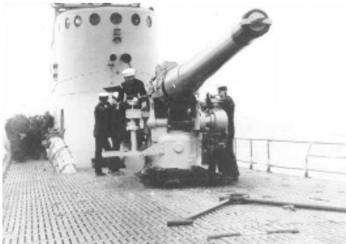
USS V-4 (later APS-1, later Argonaut SS-166) in June 1928 showing the crew manning the forward deck gun. Argonaut and her two sister-ships were the only three submarines equipped with two of the massive 6"/53 guns. Note the ammunition scuttle at left and the bipod barrel support in the foreground.
